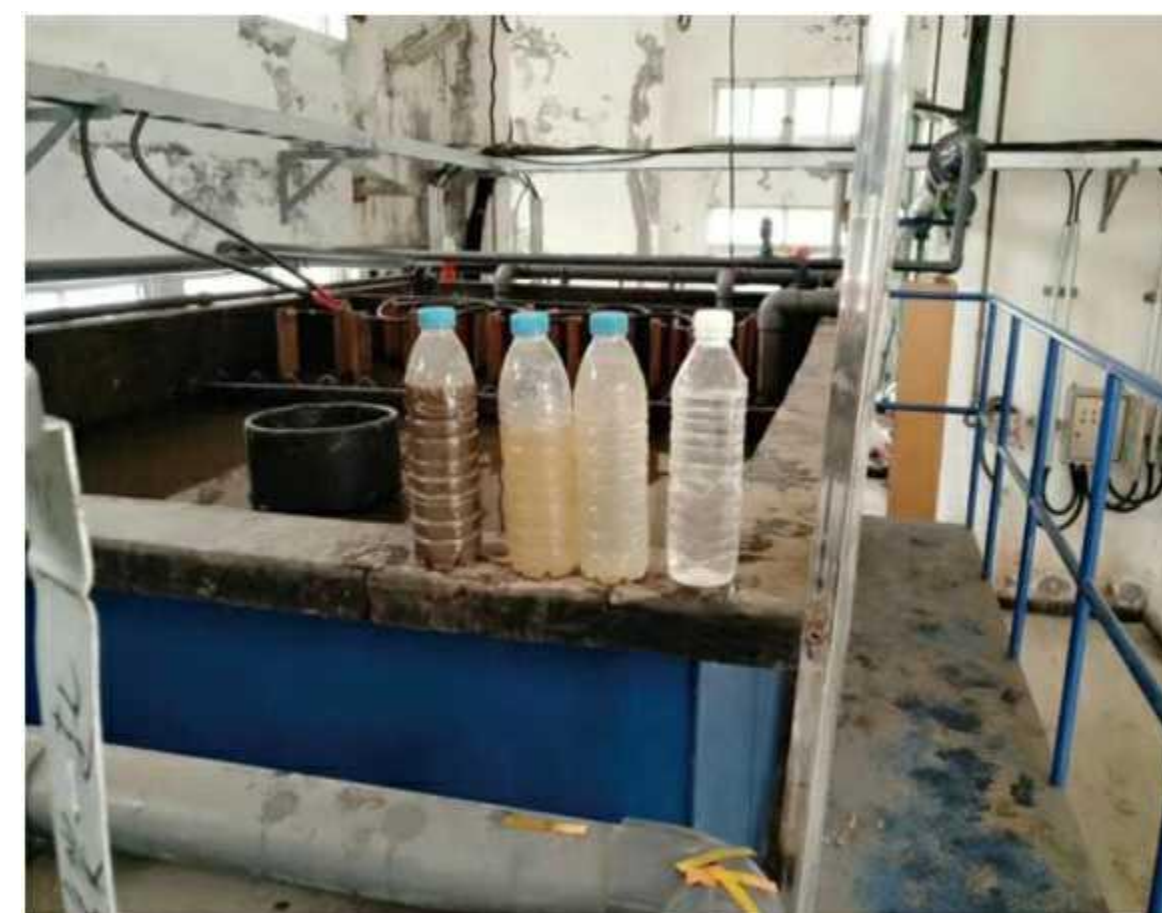
贵州某电厂脱硫废水 Desulfurization wastewater from a power plant in Guizhou
